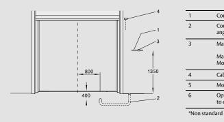
Optional safety switch on sectional door to disable leveler when door is closed\*
