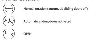
When the switch is set to "automatic sliding doors" position, the revolving door rotates to its emergency position and stops.
