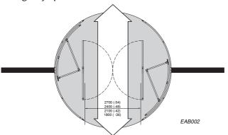
When power failure occurs, the door runs by battery to the emergency position. The lock for the escape doors, centre double swing door panels are released and can be manually broken out and give a clear evacuation path through the centre. The escape doors have to be manually closed after use. When closed, and mains is restored or the fire alarm system no longer indicates an emergency, the door will resume normal operation.
