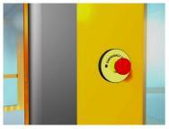
In case of an emergency, door rotation can be stopped by pressing the Emergency stop button. To reset the door to normal rotation after the emergency situation has ceased, *Section Start up after power failure, fire alarm or other status codes on page 20*. The functionality of the emergency stop buttons shall bee tested once a year.
