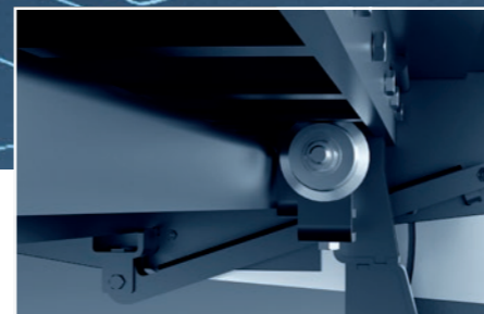
3. Dual lip guide rollers deliver smooth, precise movement during extension and retraction
