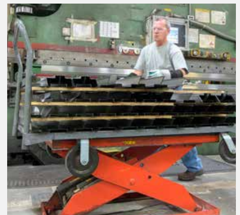
Lifting equipment adjusts working height to a comfortable level to prevent the operator from having to bend over.
