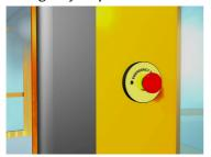
In case of an emergency, door rotation can be stopped by pressing the Emergency stop button. To reset the door to normal rotation after the emergency situation has ceased, Section Start up after power failure, fire alarm or other status codes on page 24. The functionality of the emergency stop buttons shall be tested once a year.
