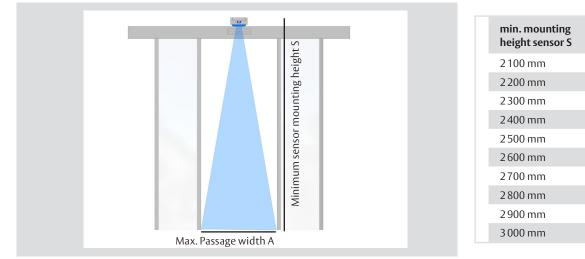
The mounting height of the sensor depends on the passage width A of the door. Please note: The passage width defines the minimum sensor installation height.
