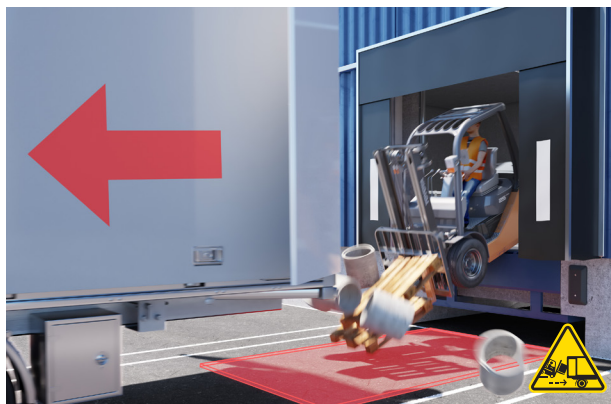
When a truck pulls away from the dock prematurely, it can have potentially fatal consequences for forklift operators or people working in the trailer or around the loading bay.
