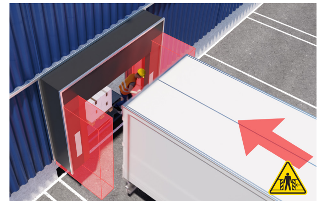
When vehicles back up to a docking bay, people standing or working around the door opening can be pinned against the loading bay entrance or hit by falling loads.
